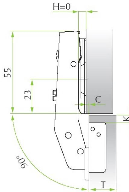
Table to determinate the minimum distance A so that a door with T thickness can open without protrusion from the cabinet and without interfering with adjacent doors.
